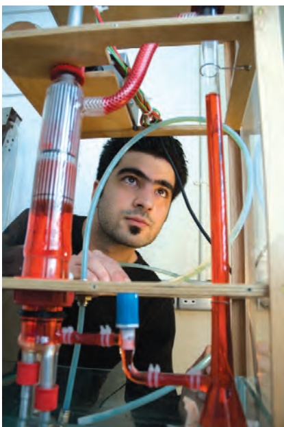
Christos Markides demonstrates the NIFTE heat pump with no moving parts
