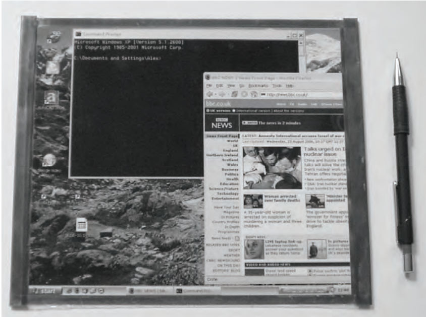
A mocked-up flexible display supported on one of Keith's morphing structures
