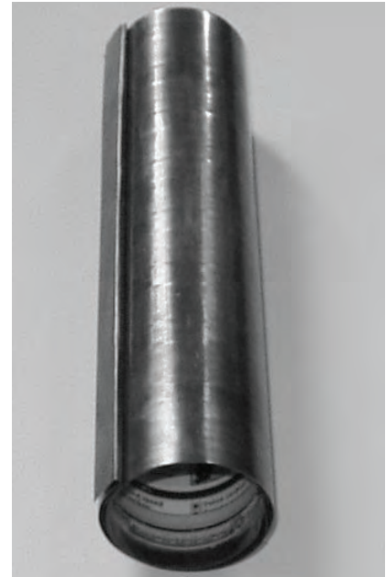
The display coiled up into a self-locking tube
