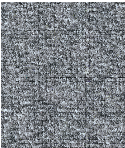
Example of a hologram as displayed on an LCoS microdisplay from the CAPE ViHPS Project. The pixels are coloured black and white to represent different phase values. The microdisplay is actually totally transparent. Photo courtesy of Jamie Christmas.
